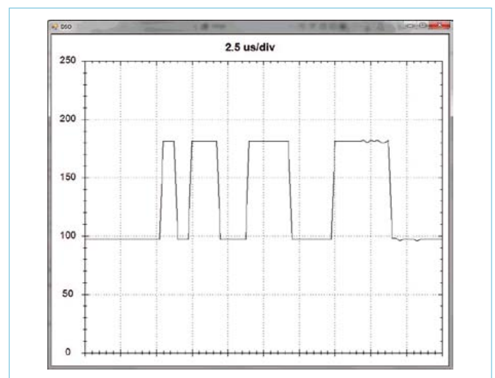
Figure 1. A 1-2-3-4- \mu s pulse train shown on the Piccolo DSO at 4 Msa.
