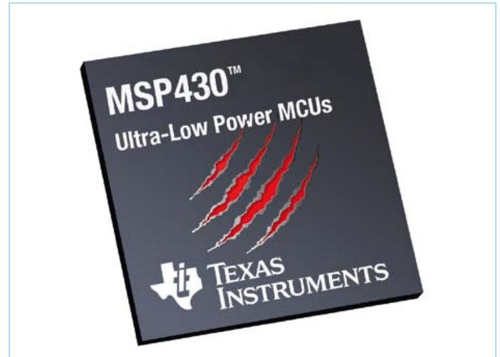
Photo 5. Named after X-Men character Wolverine, the new MSP430 from Texas Instruments features less than 100 \mu A/MHz active power consumption.
